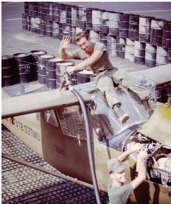
ABOVE: Two Catkiller crew chiefs work on a Birddog at Marble Mountain. The aircraft is situated within a revetment made with fifty-gallon drums filled with sand to protect it against enemy mortar attacks. (Courtesy Raymond G. Caryl)
